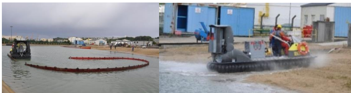
Figure 4. Tests at Cedre: towing boom in trawling configuration and U-turn on beach
