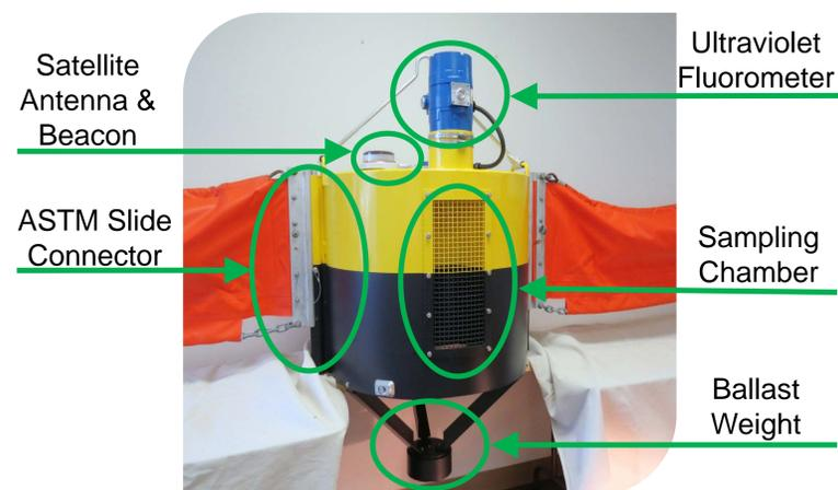
Figure 1. Exterior system components
