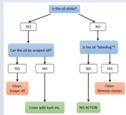
Decision-making scheme for the assessment of remediation need. (Adapted from Assessment criteria for how "clean" is "clean" in a sustainable society? Oil- and chemical spills, IVL 2007)
