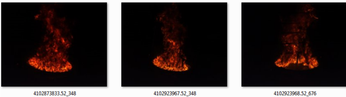
Figure 4. Side view of burning ANS
