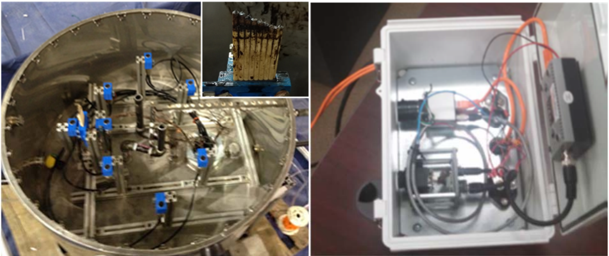
Figure 8: Acoustic transducers and thermocouples mounted inside the 70 cm diameter burn chamber and the camera enclosure.
