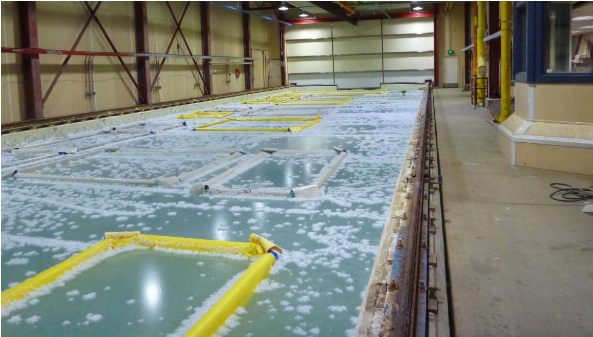
Figure 1. Hoop setup at CRREL test basin for oil in and under water detection experiments.
