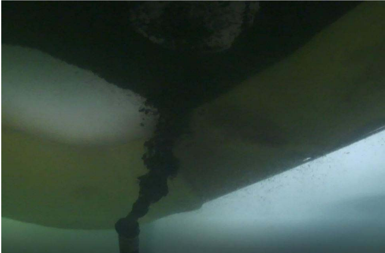
Figure 8: Subsurface image of ANS oil as it is injected into a containment hoop.
