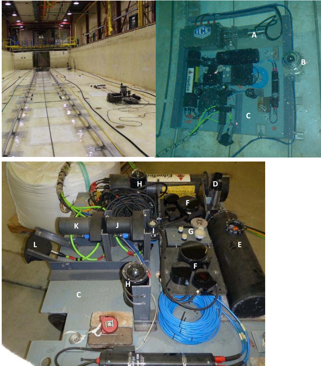
Figure 3. Top left, the rail system with the chain between the rails run down the center of the tank. Fixed sensors can be seen on the right side of the image. Top right, the sensor plate mounted to the carriage underwater. (A) The servo motor, (B) CRREL camera system on the carriage, and (C) the instrument plate. Bottom, The instrument plate out of the water. (D) Trios spectral radiance and irradiance sensors, (E) EIC Labs scanning laser fluorosensor, (F) broadband acoustic transceivers, (G) narrow band acoustic transceivers, (H) low light camera, (I) light source for the cameras, (J) Norbit 400 kHz multibeam sonar, (K) Norbit 200 kHz multibeam sonar, (L) Norbit FLS.
