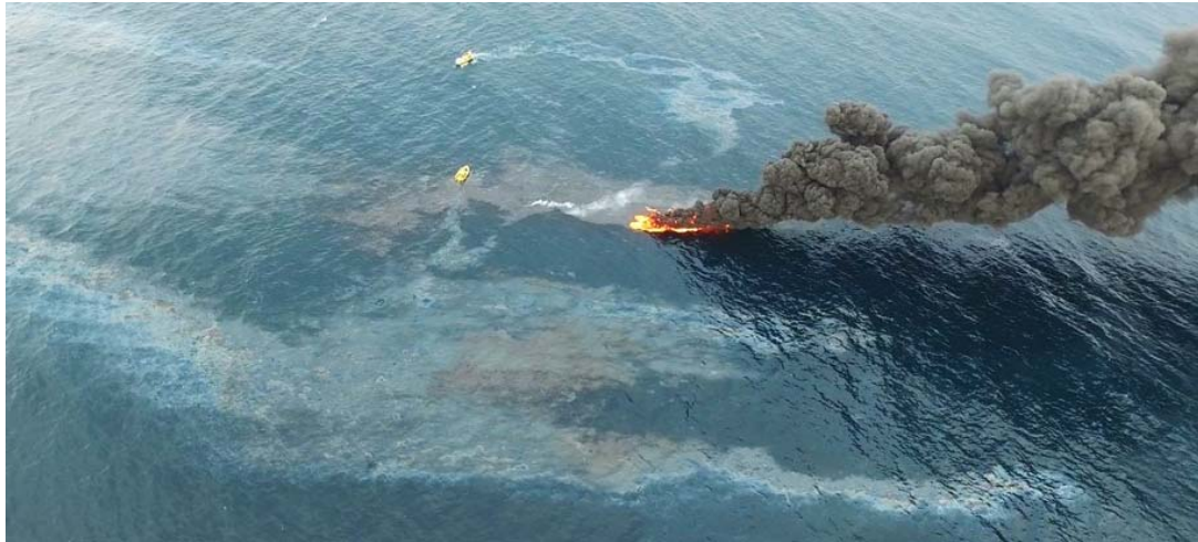
Figure 11. Ignition of herded portion of HISB 4.3 slick
