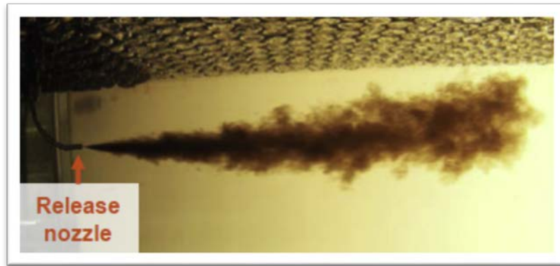
Figure 4. Example oil droplet "puff" under synthetic ice. The release nozzle on the left side is calibrated such that the amount of oil and the droplet size distribution for the "puff" is known.
