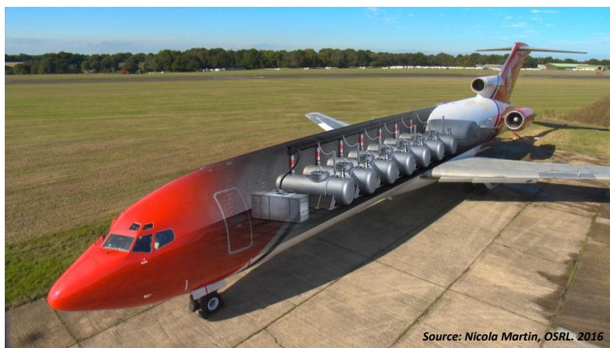
Figure 1 - Graphic Representation of the TERSUS System installed in the Boeing 727-2S2F (RE).
