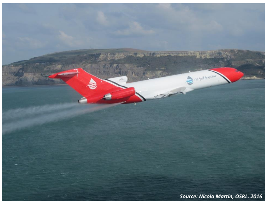
Figure 2 - G-OSRA during a spraying exercise (water spraying, in this instance).
