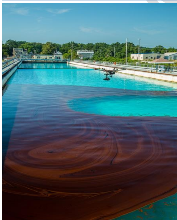
Figure 5: "Streaky" destabilized emulsion, waves off.
