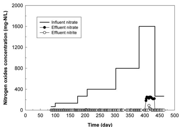
**Figure 3** Nitrogen oxides concentration with operational time
