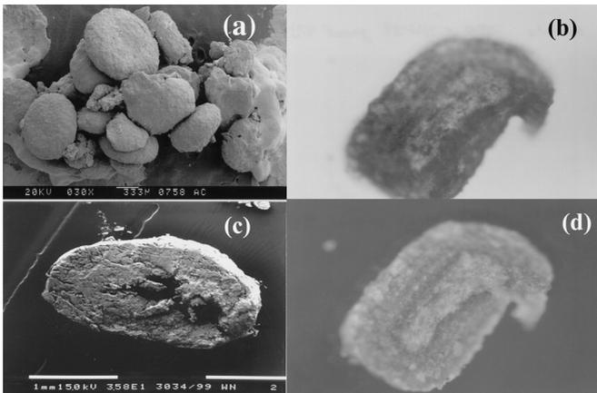
**Figure 5** Microscopy of granules (a) scanning electron microscope of agglomerated granules; (b) section of granules under light microscope; (c) scanning electron microscope of hollow granule at the top of the reactor; (d) section of granules under the epi-fluorescent excitation
