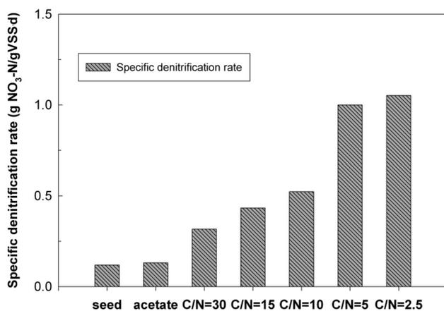
**Figure 8** Specific denitrification rate with various operating conditions
