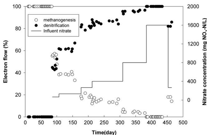
**Figure 6** Percentage of electron flow by methanogenesis and denitrification
