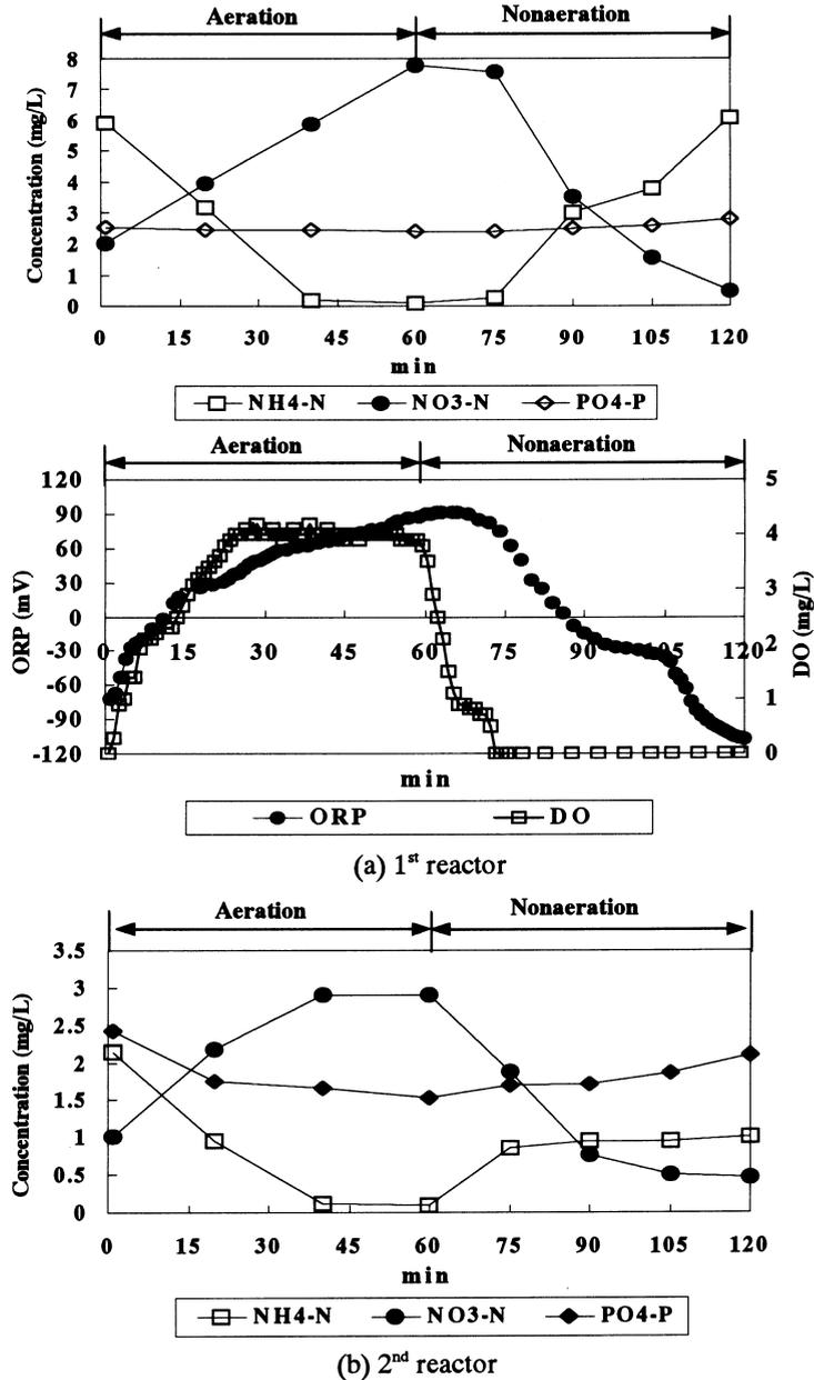
Figure 5 Water quality variation in SMBR during one cycle operation
