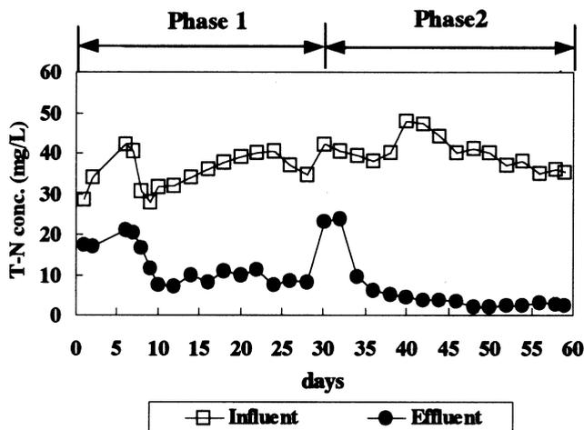
Figure 3 Daily observation of TN removal during operation period of SMBR
