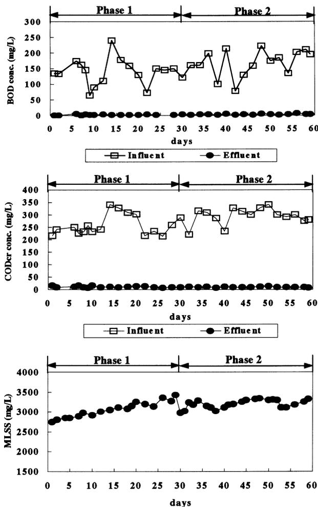
**Figure 2** Removal of organic matter and variation of MLSS concentration in SMBR
