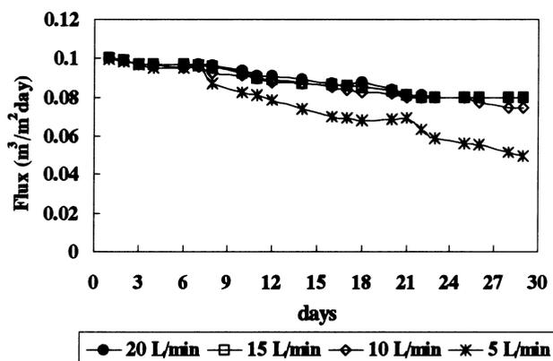
Figure 7 Flux decline at various airflow rates at suction pressure 10 kPa
