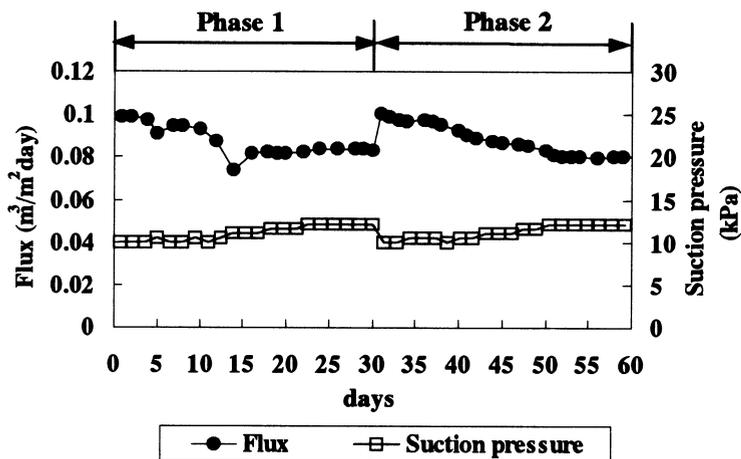
Figure 6 Variation of flux and suction pressure in SMBR
