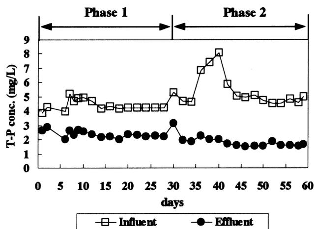
Figure 4 Daily observation of TP removal during operation period of SMBR
