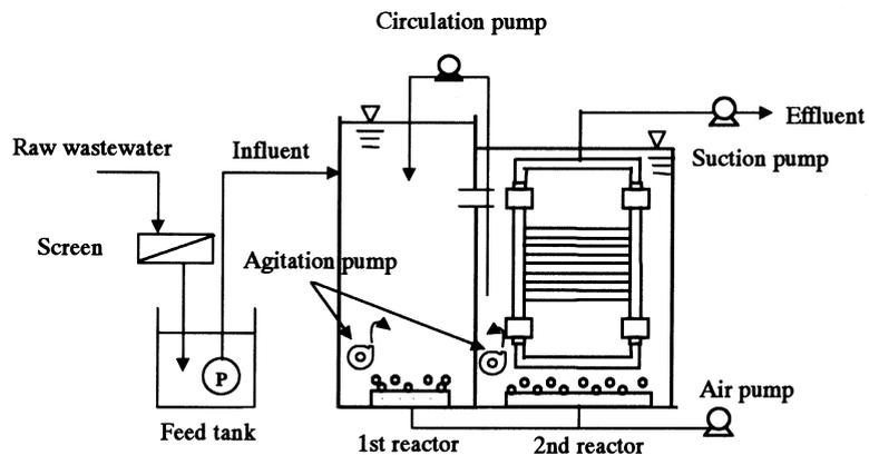
**Figure 1** Schematic diagram of the membrane bioreactor for domestic wastewater
