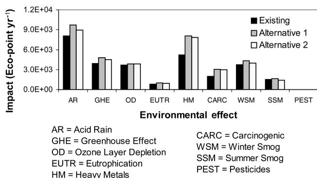
**Figure 5** | Environmental effect profile for an annual production of 70 and 83 million  $\text{m}^3$  respectively for the existing and the future alternative treatment schemes.
