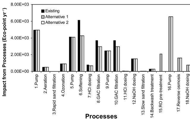
**Figure 4** | Impact from the individual process steps in the existing and future treatment schemes.
