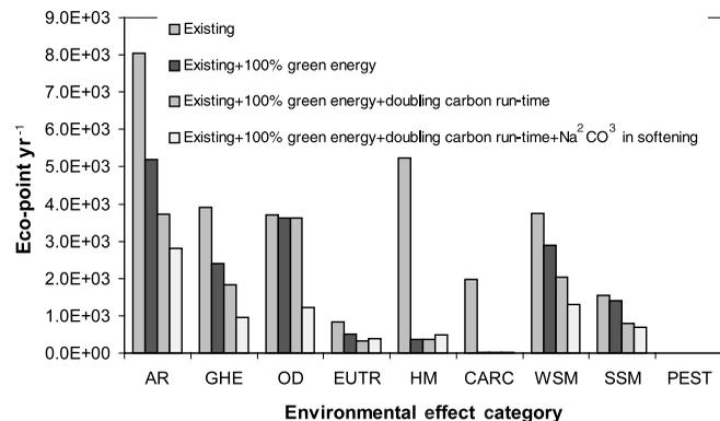
**Figure 9** | Environmental effect profiles of the existing treatment scheme before and after impact reduction.
