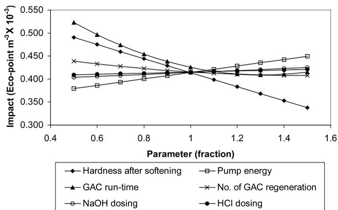
**Figure 6** | Environmental impact as a function of the values of six process parameters in the existing treatment scheme.
