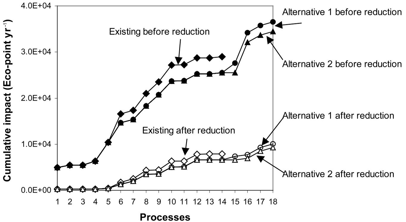
**Figure 8** | Cumulative eco-point profiles of the existing and the two alternative schemes before and after implementing the impact reduction options: using 100% green energy, doubling the carbon run-time and using Na<sub>2</sub>CO<sub>3</sub> in the softening process.
