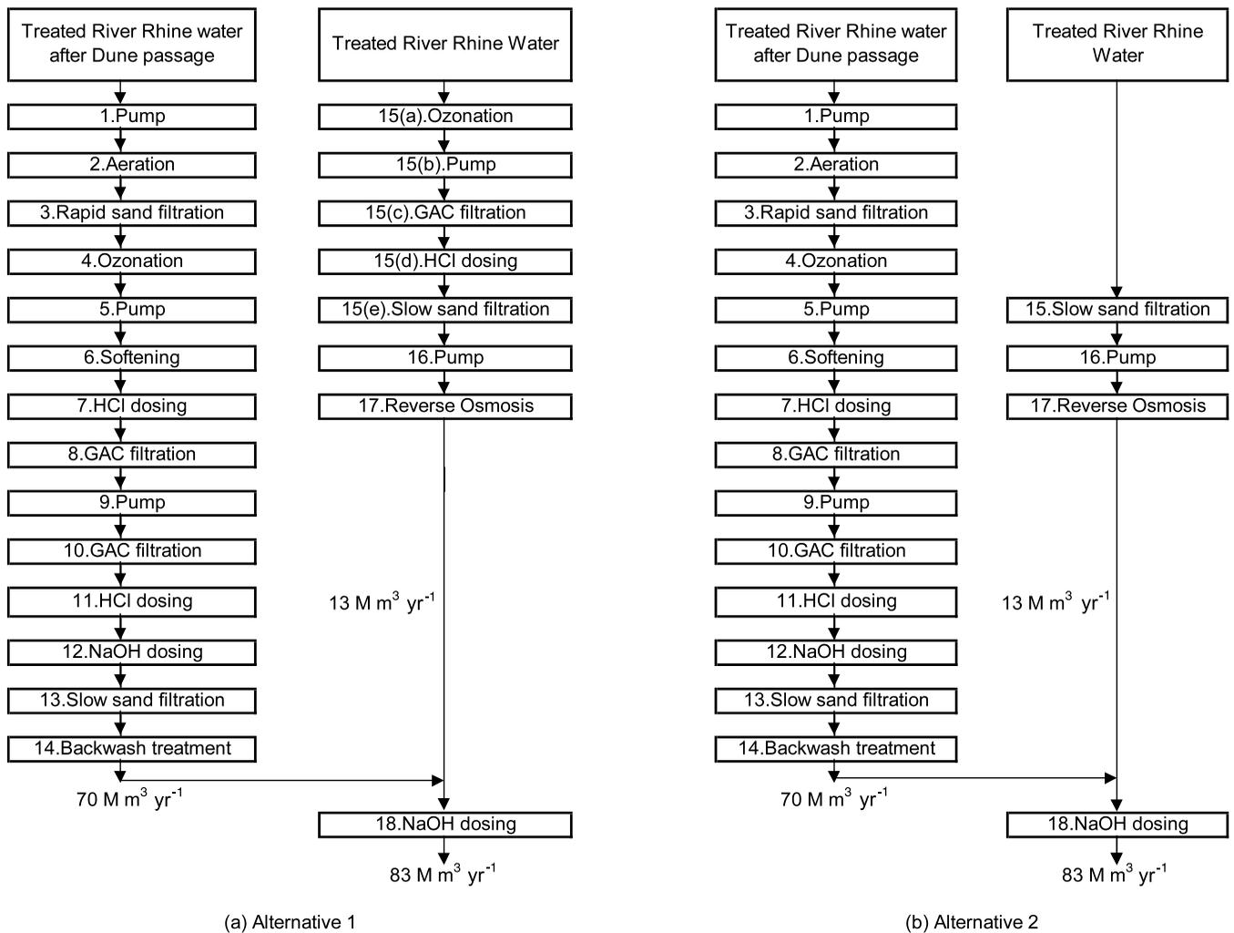
**Figure 2** | Alternative treatment schemes for annual production of 83 million m<sup>3</sup> water. (a) With expansion treatment line consisting of ozonation, GAC and slow sand filtration, and (b) with expansion treatment line consisting of slow sand filtration only for reverse osmosis pretreatment.
