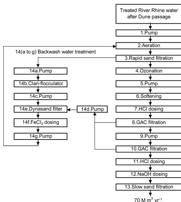
**Figure 1** | Flow chart of the existing treatment scheme of the Leiduin plant (Van der Hoek & Groot 1999).
