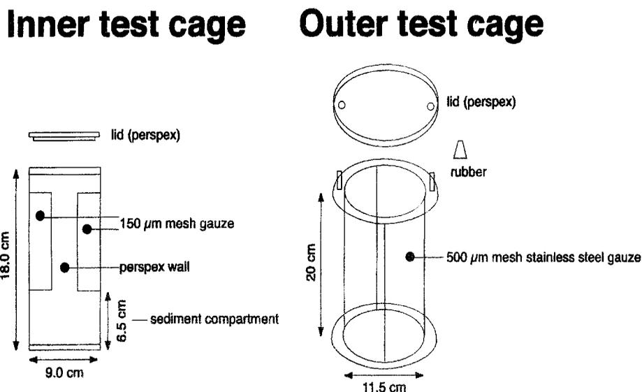
**Figure 1.** Diagram of the field cage used for in situ bioassays with *C. riparius*.
