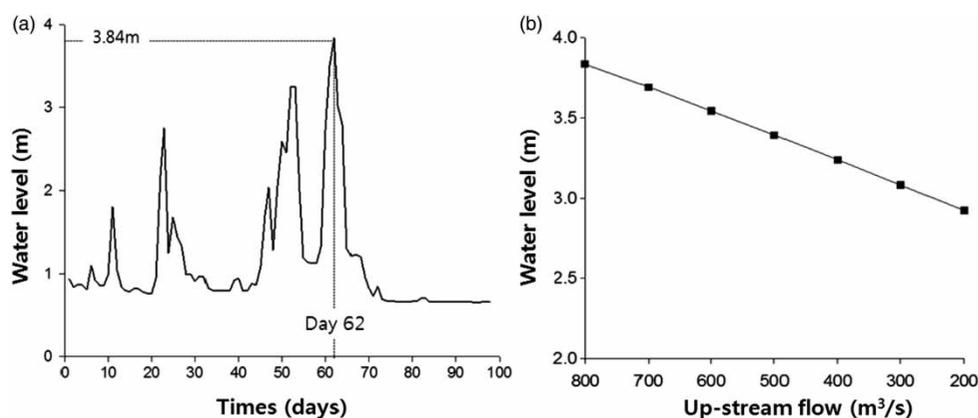
**Figure 6** | Example illustrating the decision operation of the upstream water infrastructure at point 1 of the Geum River: (a) prediction of the 1-day ahead water level; (b) estimated relation between upstream flow (day 61) and downstream water level (day 62).
