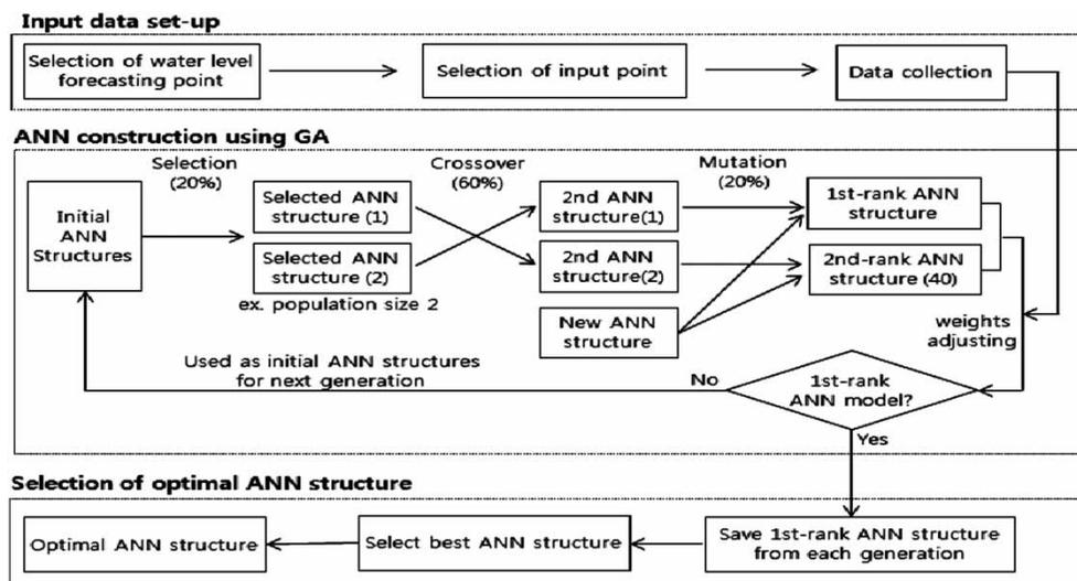
**Figure 3** | Overall model construction procedure in this study.
