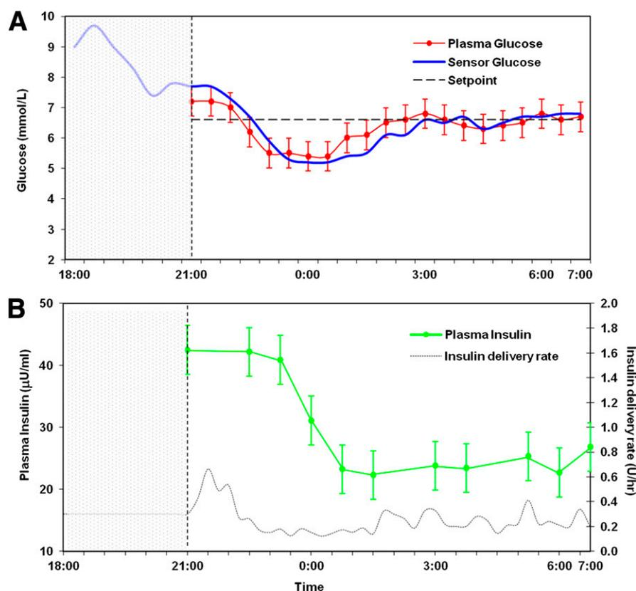
**Figure 2**—Summary of the overnight closed-loop experiment in the eight participants. The open-loop period is represented by the shaded area. An evening meal and prandial bolus were administered at 1800, and the closed-loop mode commenced at 2100. A: Sensor glucose (blue) closely tracks plasma glucose (red). B: Pump delivery rates are represented as a black dashed line, and hourly plasma insulin measurements are represented in green.
