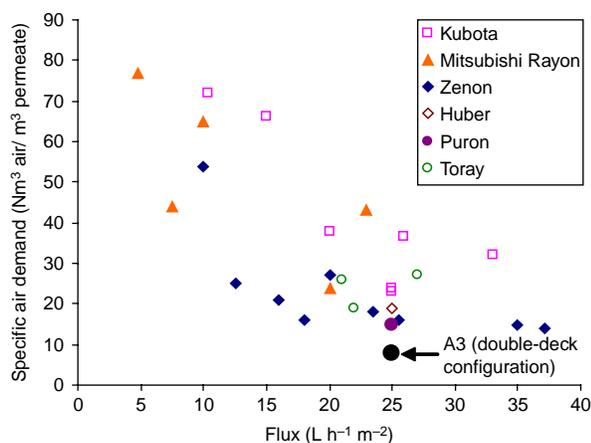
**Figure 6** | SADp in function of the net flux for various MBR plants (Judd 2007) and the pilot unit of Anjou Recherche, using A3 Water Solutions technology.
