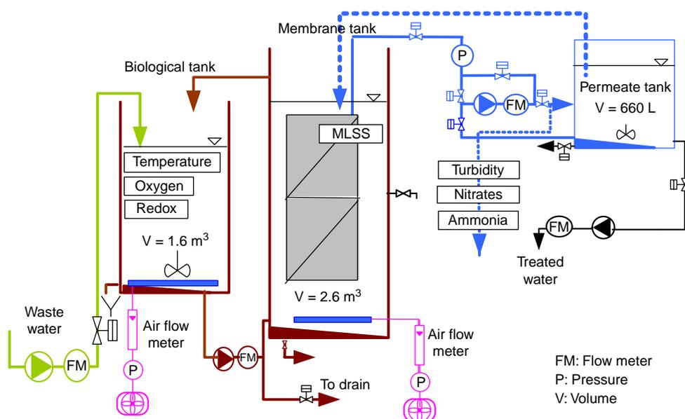
Figure 1 | Pilot plant configuration.
