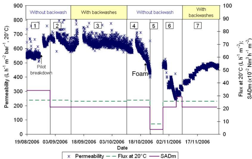
**Figure 3** | Comparison of the operation with and without backwashes.
