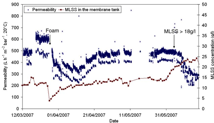
**Figure 4** | Operation at a net flux of  $25 \text{ L h}^{-1} \text{ m}^{-2}$  for a SADm of  $0.2 \text{ Nm}^3 \text{ h}^{-1} \text{ m}^{-2}$  with peak flows and MLSS concentration from 4 to 24 g/l.
