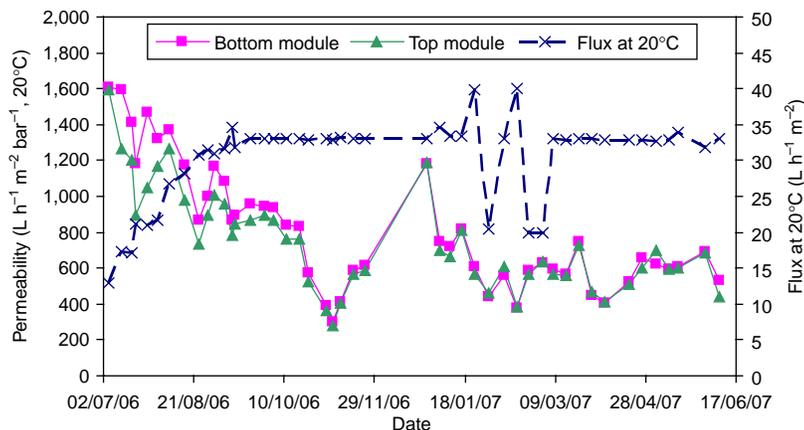
**Figure 5** | Evolution of the permeability of each module.
