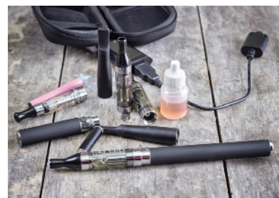
E-cigarettes are battery-operated devices that vaporize nicotine-containing fluid instead of burning tobacco like traditional cigarettes.
