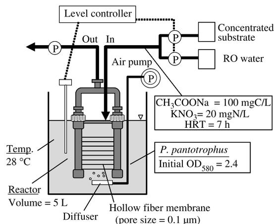
**Figure 1** Experimental unit of membrane nitrogen removal process
