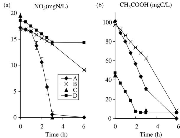
**Figure 2** Temporal changes of (a) nitrate and (b) carbon under high bacterial density
