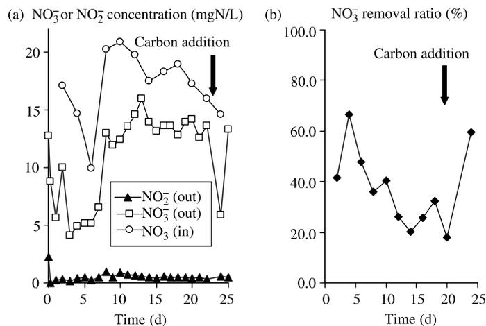
**Figure 3** Nitrogen removal during continuous operation (a) temporal changes in concentrations (b) temporal changes in nitrate removal ratio
