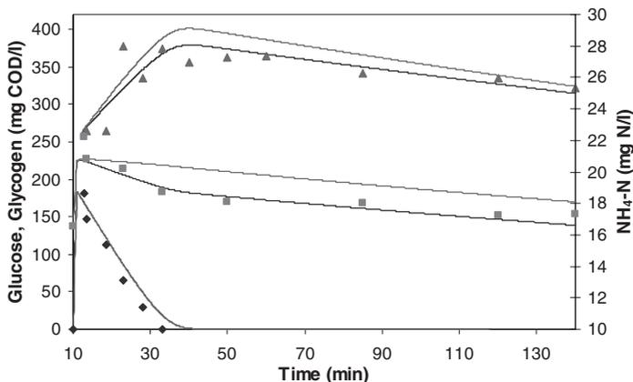
**Figure 3** Experimental data for ◆ glucose, ▲ glycogen and ■ ammonia and the model simulation results for — ASM3 and — modified ASM3
