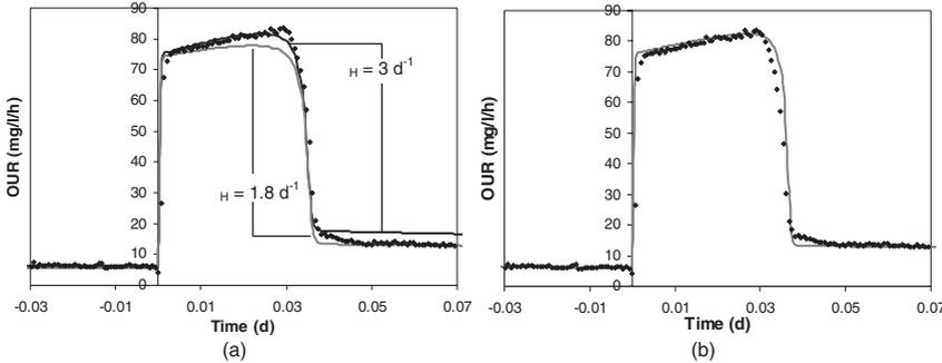
**Figure 2** OUR simulations performed using (a) ASM3 for two different growth rates and (b) modified ASM3
