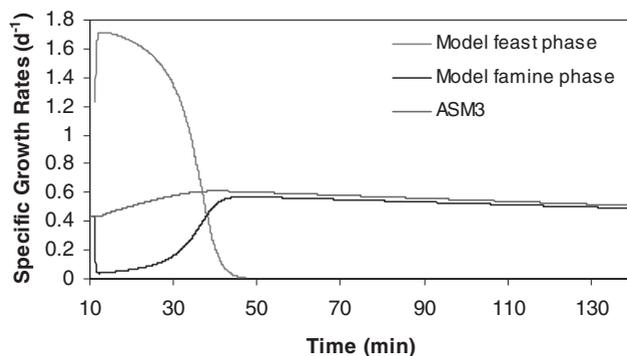
**Figure 5** Specific growth rates obtained for proposed model and for ASM3
