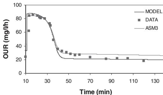
**Figure 4** OUR data and the model simulation results for proposed model and for ASM3
