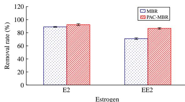
**Figure 6** | Comparison of E2 and EE2 removal in MBR and PAC-MBR sludge.
