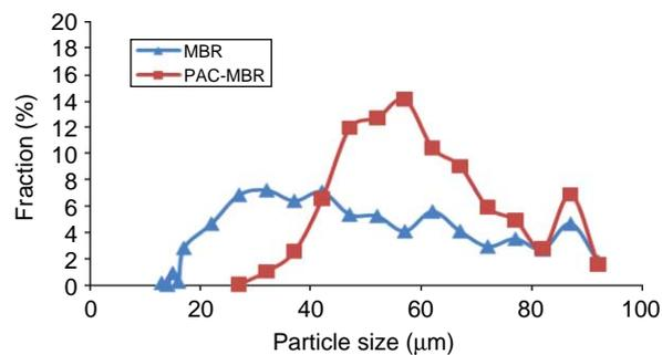
**Figure 5** | Comparison of particle size distribution between MBR and PAC-MBR sludge.
