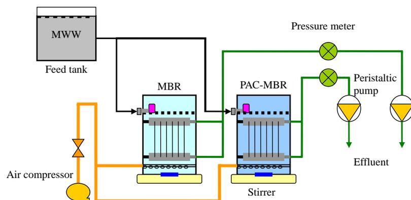
**Figure 1** | Schematic of the bench-scale MBR and PAC-MBR.
