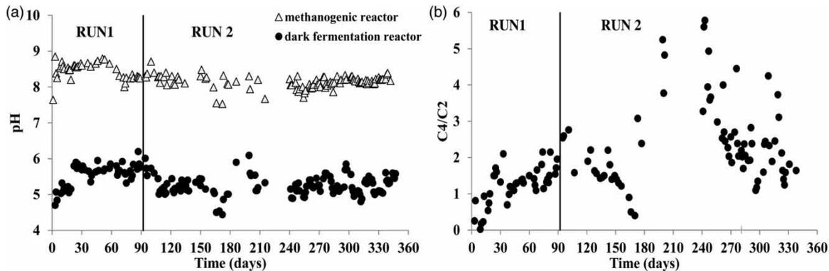
**Figure 3** | (a) pH in the dark fermentation reactor; (b) butyrate and acetate ratio (C4/C2) in the dark fermentation reactor.
