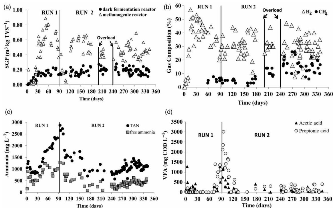
**Figure 2** | (a) SGP of both reactors; (b) gas composition of the dark fermentation reactor; (c) total ammonia nitrogen (TAN) and free ammonia of methanogenic reactor; (d) acetate and propionate of dark fermentation reactor.
