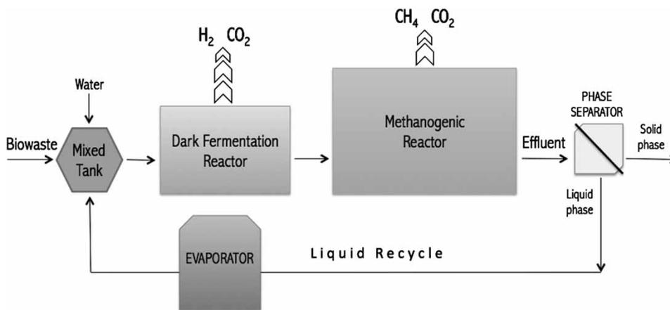
Figure 1 | Flow scheme of two-stage technology adopted for bio-hythane production.
