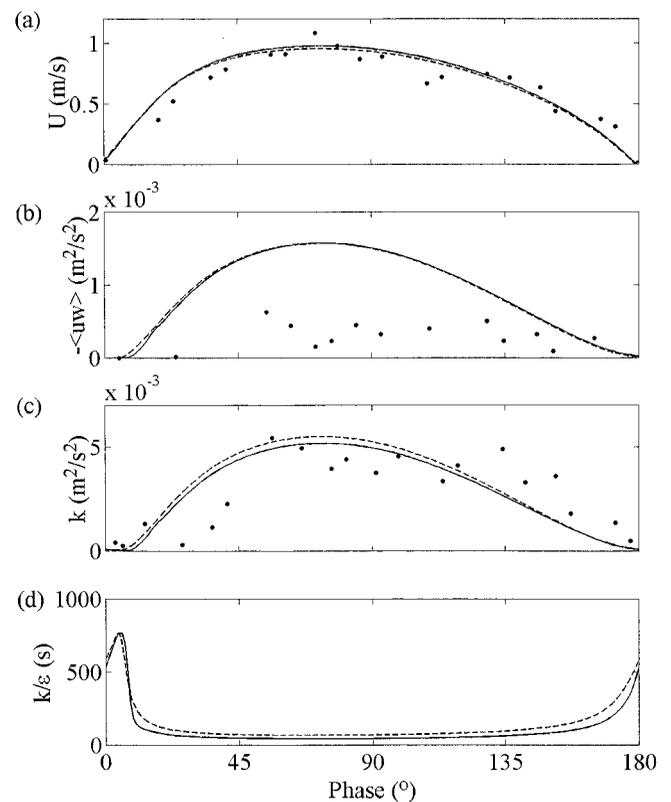
**Figure 2** | Cyclic variations in the Elbe estuary at 1.9 m above the bed. (a) Velocity, (b) Reynolds stress, (c) turbulent kinetic energy, (d) turbulence timescale. • Data of Schröder (1987), —  $k-\epsilon$  model, ---  $k-l$  model.
