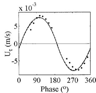
**Figure 9** | Cyclic variation of friction velocity in comparison with the present UMTF data. •Data, —  $k-\epsilon$  model, ---  $k-l$  model.
