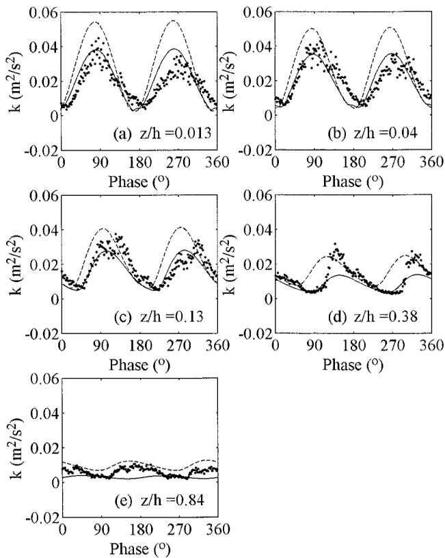
**Figure 5** | Cyclic variation of turbulent kinetic energy in comparison with Case 13 of Jensen *et al.* (1989). •Data, —  $k-\epsilon$  model, ---  $k-l$  model. The experimental data for  $k$  are approximated by  $k' = 1.3(u^2 + w^2)/2$ .
