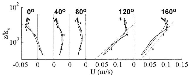
**Figure 8** | Velocity profiles at various phase positions in comparison with the UKCRF data of Lloyd *et al.* (1997). •Data, —  $k-\epsilon$  model, ---  $k-l$  model, - · - semi-logarithmic fit to data.
