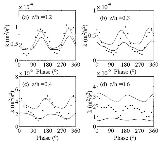
**Figure 12** | Cyclic variation of turbulent kinetic energy in comparison with the present UMTF data. •Data, —  $k-\epsilon$  model, ---  $k-l$  model. The experimental data for  $k$  are approximated by  $k' = 1.3(u^2 + w^2)/2$ .
