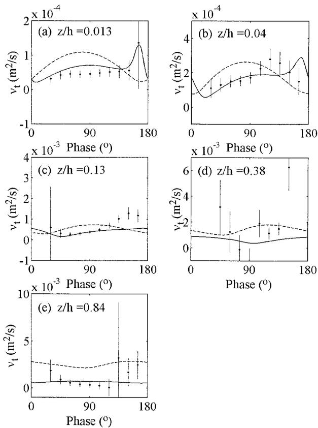
**Figure 6** | Cyclic variation of eddy viscosity in comparison with Case 13 of Jensen *et al.* (1989). •Data, —  $k-\epsilon$  model, ---  $k-l$  model. The vertical lines give a measure of the uncertainty in the experimental points.
