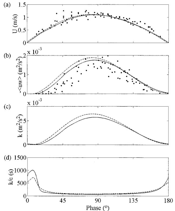
**Figure 1** | Cyclic variations in the Jade estuary at 2.14 m above the bed. (a) Velocity, (b) Reynolds stress, (c) turbulent kinetic energy, (d) turbulence timescale. •Data of McLean (1983), —  $k-\epsilon$  model, - -  $k-l$  model.
