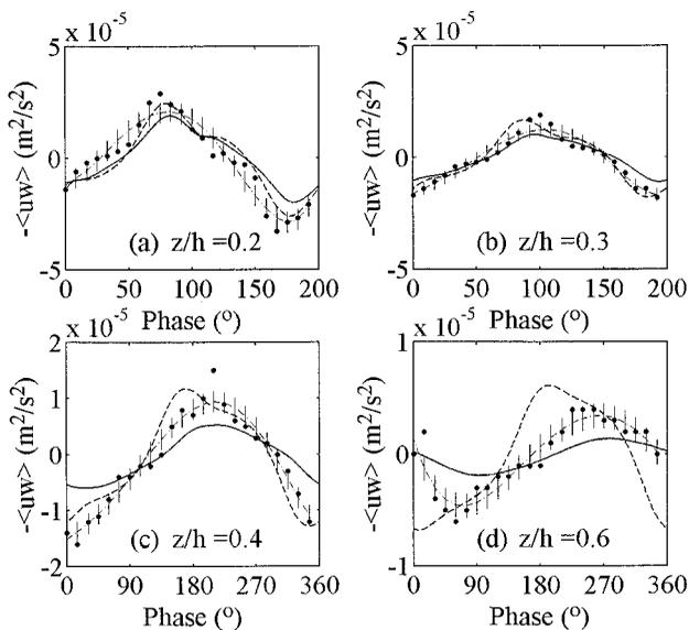
**Figure 11** | Cyclic variation of Reynolds shear stress in comparison with the present UMTF data. •Data, —  $k-\epsilon$  model, ---  $k-l$  model, -.- polynomial fit to data. The vertical lines give a measure of the uncertainty in the fit to data.
