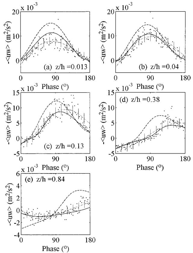
**Figure 4** | Cyclic variation of Reynolds stress in comparison with Case 13 of Jensen *et al.* (1989). •Data, —  $k-\epsilon$  model, ---  $k-l$  model, - - - polynomial fit to data. The vertical lines give a measure of the uncertainty in the fit to data.
