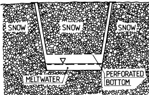
Fig. 6. Snow evaporimeter used at the University of Luleå. Surface area = 0.314 m<sup>2</sup>.
