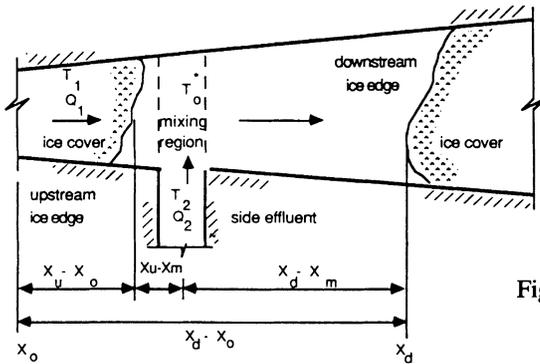
Fig. 2. Channel configuration with various geometrical locations.
