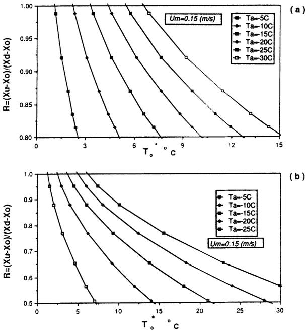
Fig. 4. Calculated ice suppression ratio for  $u = 0.15$  m/sec.; a) convergent flow; b) divergent flow.
