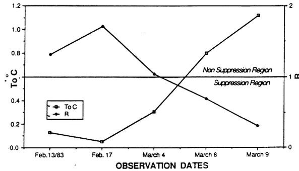
Fig. 9. Interrelation between  $R$  and  $T_0^*$  Calculated ice suppression ratio for various observation dates, (with mixing assumption).
