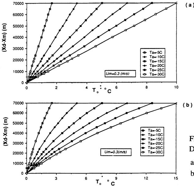
Fig. 3. Downstream ice edge locations; a) convergent flow; b) divergent flow.
