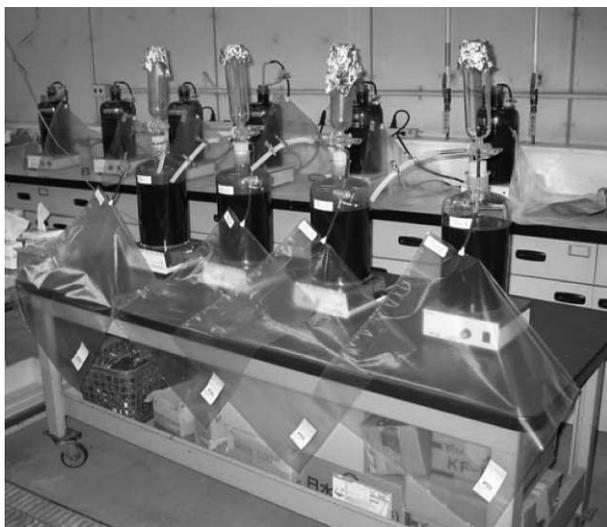
**Figure 3** Anaerobic digestion test apparatuses
