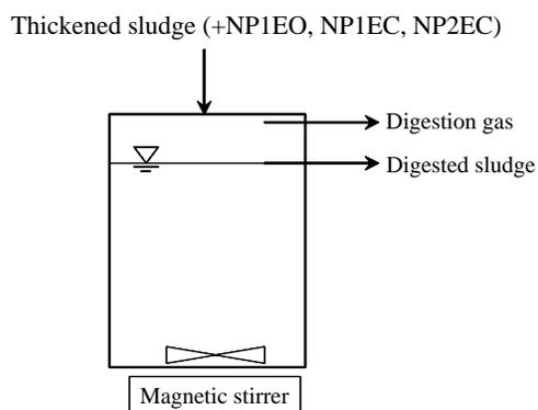
**Figure 2** Outlines of an anaerobic digestion test apparatus
