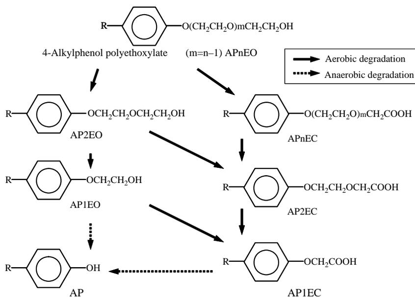
**Figure 1** Decomposition of nonylphenol polyethoxylates (based on Ahel *et al.*, 1994) AP: Nonylphenol, R: C<sub>9</sub>H<sub>19</sub>
