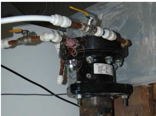
Figure 2 | Modified top end-plate to allow entry and exit of the cooling water.
