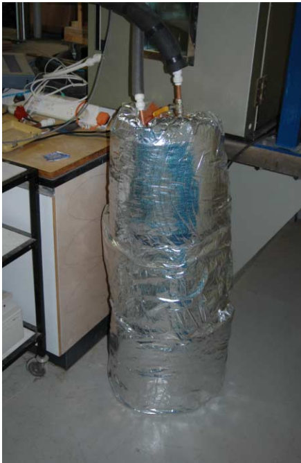
Figure 4 | General arrangement of unrestrained pipe test showing position of top end-plate and thermal insulation in place.
