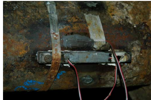
Figure 6 | Invar bar, with its surface mounted strain gauge, attached to the pipe adjacent to the measurement gauge.
