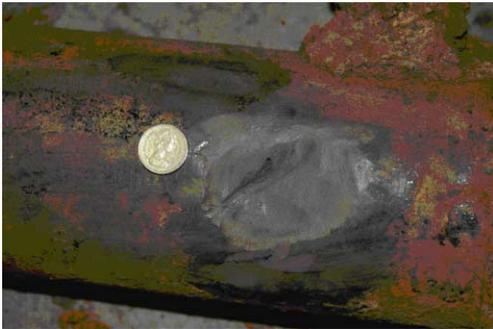
**Figure 1** | Typical surface condition of supplied cast iron pipe showing extensive graphitic corrosion of pipe wall.
