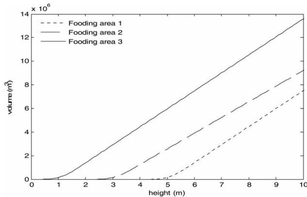
Figure 4 | Flooding areas modelling: relation between height and volume.
