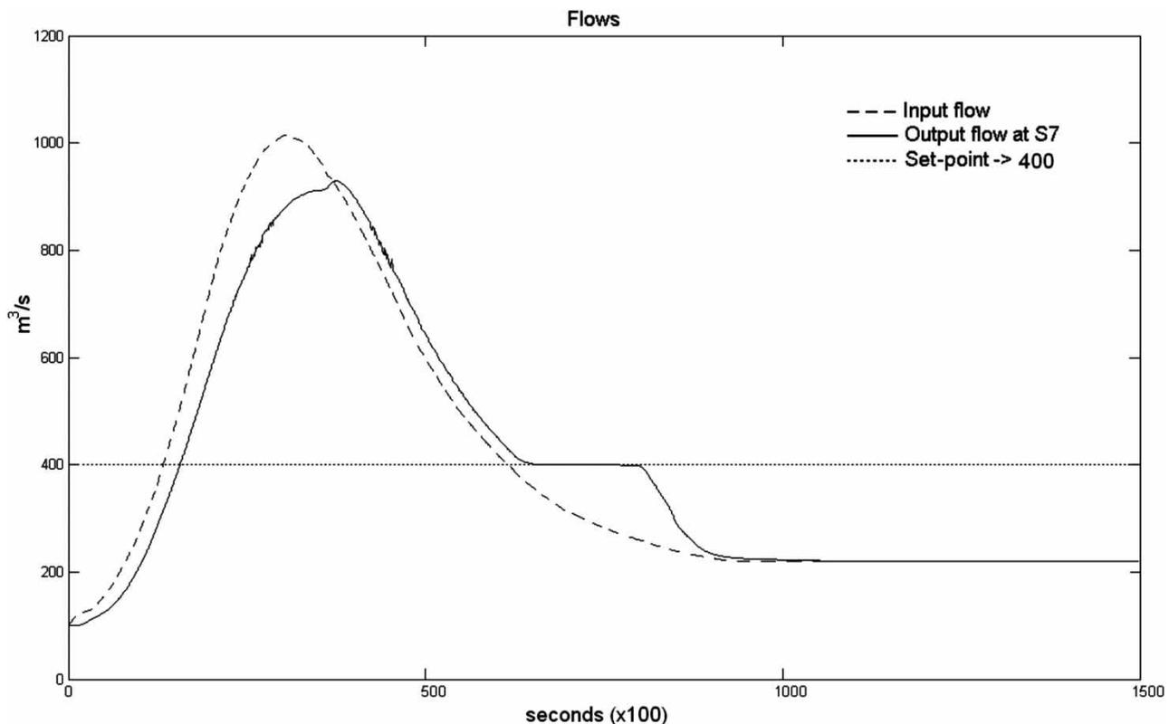
Figure 10 | Results of the indirect flow PID control strategy.
