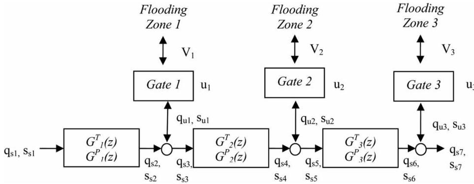
Figure 2 | Block diagram of the Ebro system.
