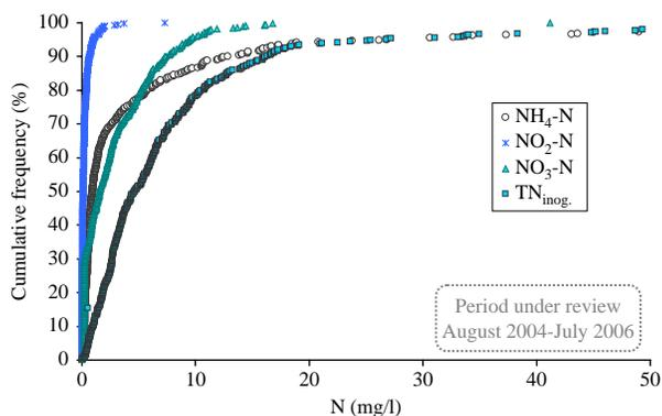
**Figure 5** | Statistic analysis of nitrogen concentrations in the effluent. Subscribers to the online version of *Water Science and Technology* can access the colour version of this figure from <http://www.iwaponline.com/wst>
