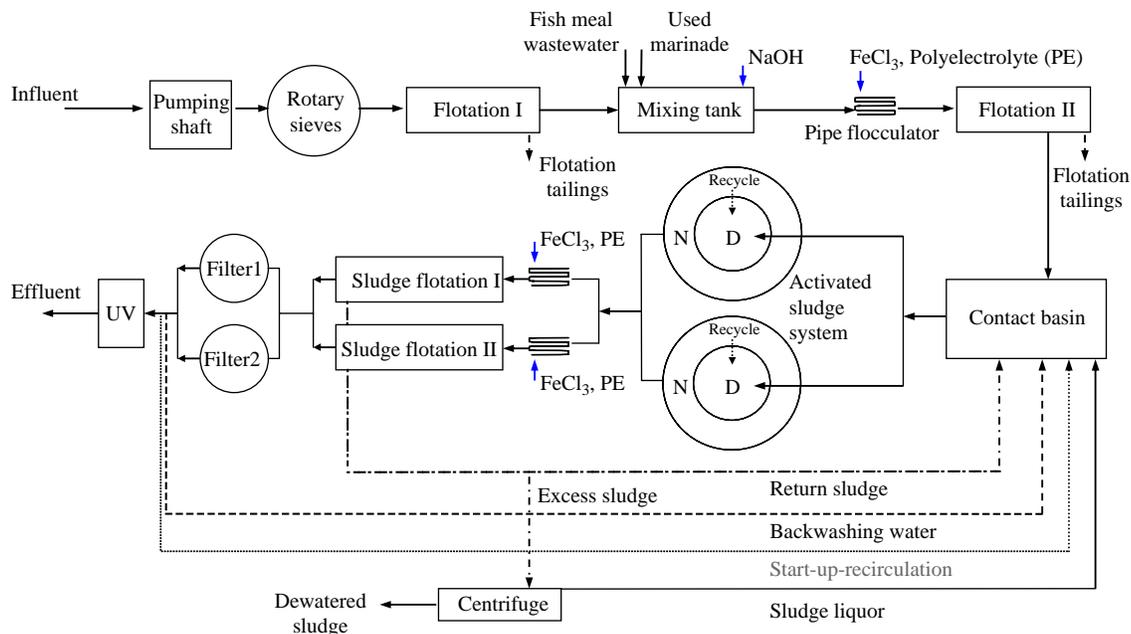
Figure 1 | Flow scheme of the wastewater treatment plant.
