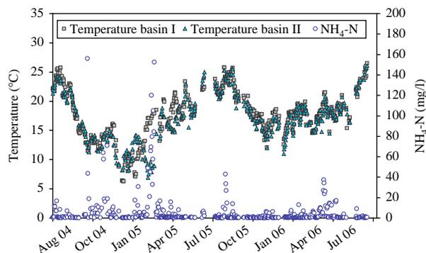
**Figure 4** | Temperature in the activated sludge basins and ammonia nitrogen in the effluent.
