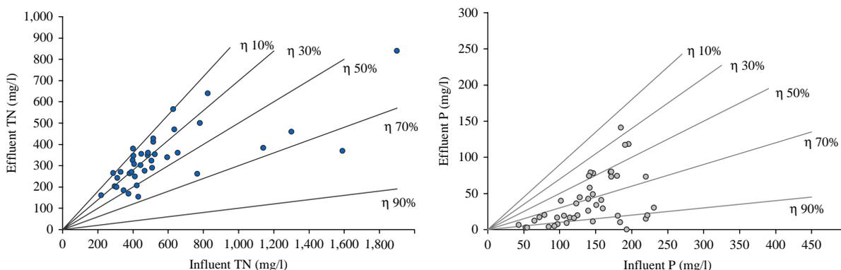
Figure 3 | Nitrogen and phosphorus removal with flotation.
