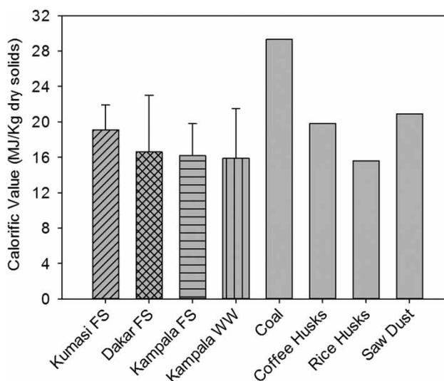
**Figure 1** | Average calorific value of raw faecal sludge from Kumasi ( $n = 11$ ), Dakar ( $n = 26$ ), and Kampala ( $n = 29$ ), and WWTP sludge from Kampala ( $n = 4$ ) compared with traditional biomass fuels (Alakangas et al. 2007).
