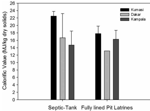
**Figure 2** | Average calorific value of faecal sludge samples from septic tanks and fully lined pit latrines in Kumasi (Septic  $n = 10$ ; PL  $n = 20$ ), Dakar (Septic  $n = 19$ , PL  $n = 1$ ), and Kampala (Septic  $n = 15$ , PL  $n = 23$ ).
