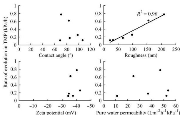
**Figure 5** | Correlation between the rate of evolution in TMPs and membrane properties.
