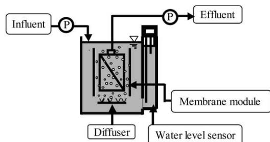
Figure 1 | Schematic diagram of laboratory-scale MBR.
