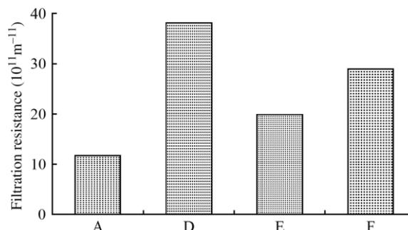
Figure 4 | Filtration resistance caused by physically irreversible fouling ( $R_{ir}$ ).
