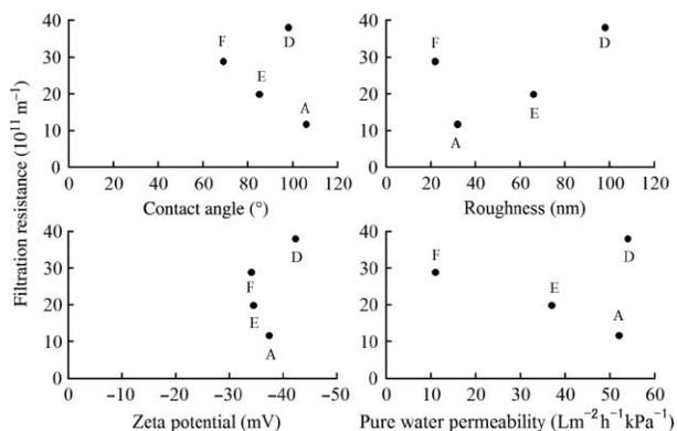
**Figure 6** | Correlation between the degree of physically irreversible fouling and membrane properties.
