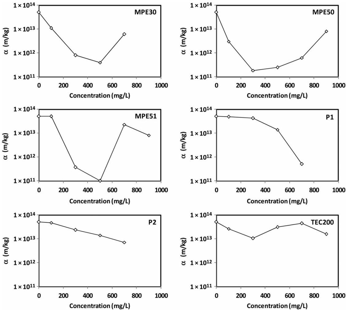
Figure 1 | Specific cake resistance of the sludge after application of different dosages of the tested flocculants.
