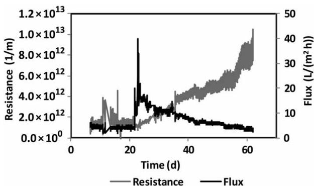
**Figure 4** | TMP and permeate flux during the operation of the AnMBR. Flocculant (MPE50) was added on day 22.
