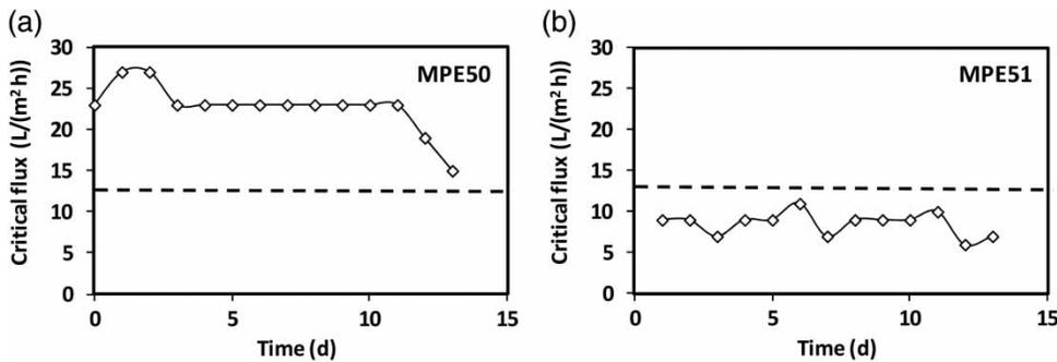
Figure 2 | Stability of the flocs formed by flocculants MPE50 (a) and MPE51 (b), expressed as evolution of critical flux. Dotted lines indicate the critical flux of the original sludge. Flocculant dosage: 300 mg/L, solids concentration: 9 g TSS/L.
