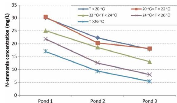
Figure 10 | Concentration of ammonia as a function of temperature ranges in the ponds.
