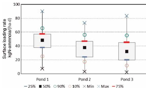
Figure 9 | Box-plot of surface loading rate of ammonia throughout the ponds.
