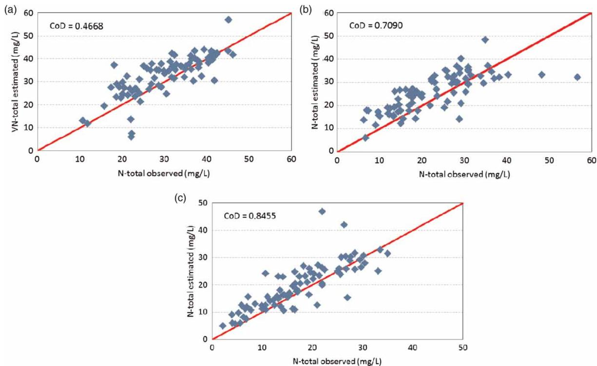
**Figure 13** | Observed values vs estimated values of total nitrogen in Ponds 1, 2 and 3, utilizing the Reed model. (a) Pond 1, (b) Pond 2 and (c) Pond 3.
