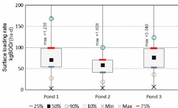
Figure 8 | Box-plot of surface loading rate of BOD throughout the ponds.
