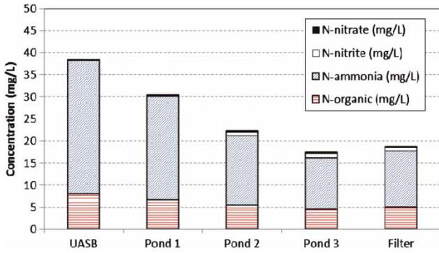
Figure 2 | Mean values of the different nitrogen fractions throughout the treatment units.
