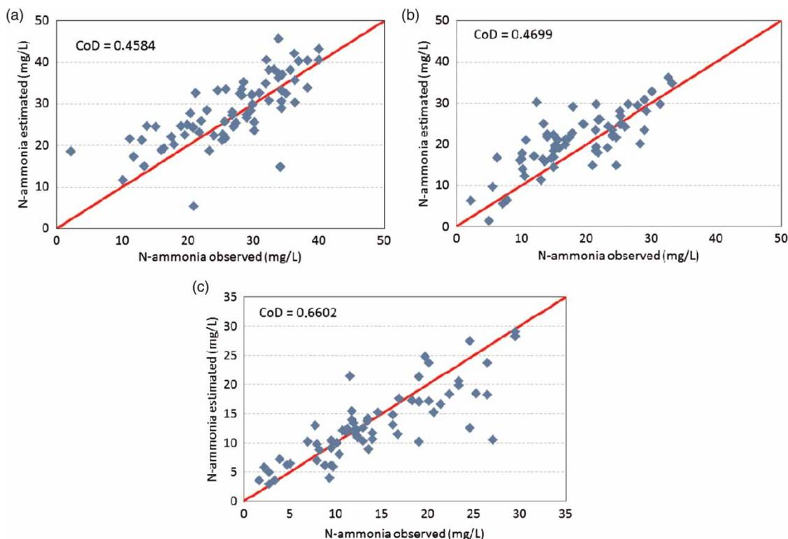
Figure 12 | Observed values vs estimated values of ammonia in Ponds 1, 2 and 3, according to the Pano and Middlebrooks model. (a) Pond 1, (b) Pond 2 and (c) Pond 3.
