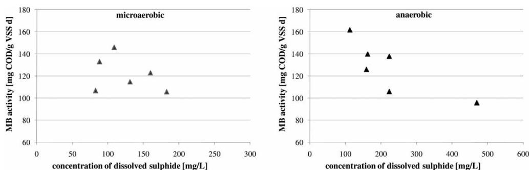
Figure 4 | Relation between specific methanogenic activity and concentration of dissolved sulfide.
