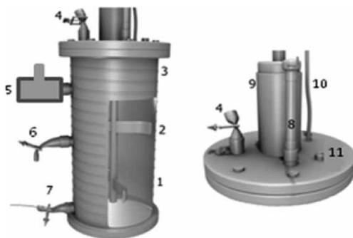
**Figure 1** | The scheme of the reactor: 1. body of reactor, 2. paddle-wheel stirrer, 3. resistance heater, 4. input pipe for substrate, 5. vessel for ORP analysis, 6. sampling point, 7. air supply, 8. thermometer, 9. water-cap, 10. biogas output to gas flow meter, 11. septum for biogas sampling.
