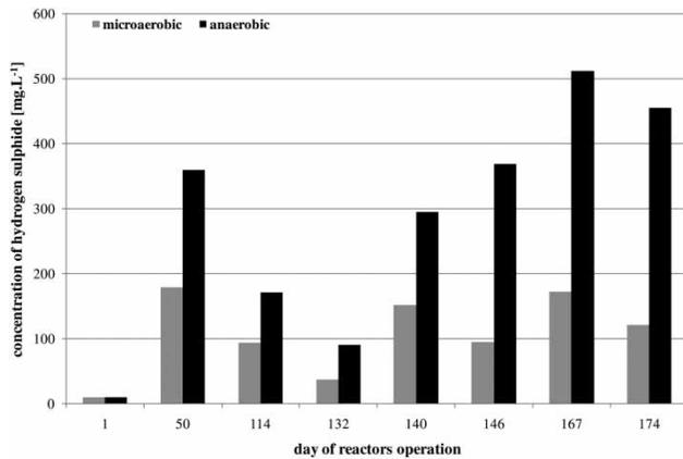
**Figure 2** | Hydrogensulphide concentration in biogas in days of methanogenic activity testing.
