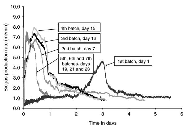
**Figure 1** | Evolution of the biogas production rate for batches during the start-up period.
