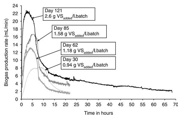
**Figure 3** | Evolution of biogas production rates at different organic loading rates.
