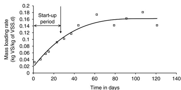
**Figure 2** | Evolution of the specific activity of the anaerobic biomass during the whole experiment.
