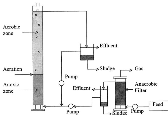
Figure 1 Schematic diagram of the submerged filters-in-series system
