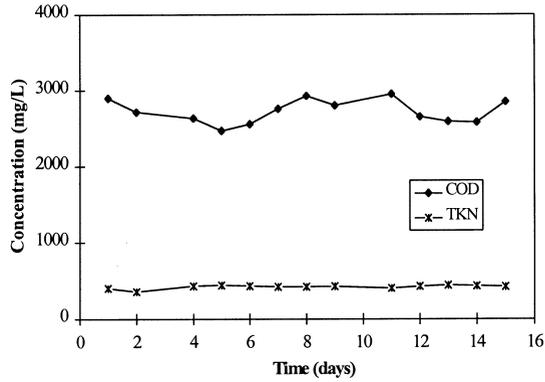
Figure 3 Concentrations of effluent after first-stage anaerobic treatment
