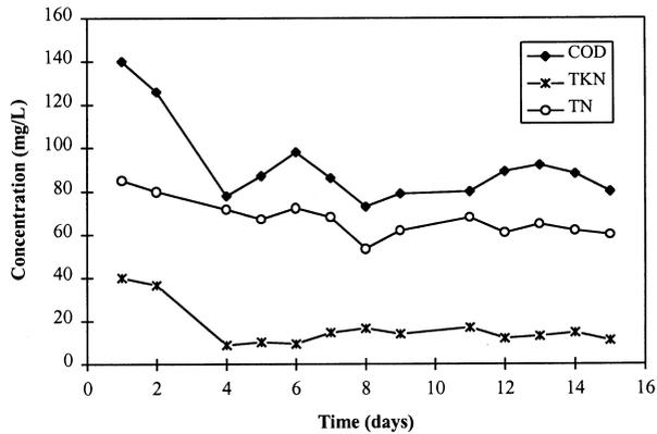
Figure 5 Concentrations of effluent after second-stage A/O filter treatment
