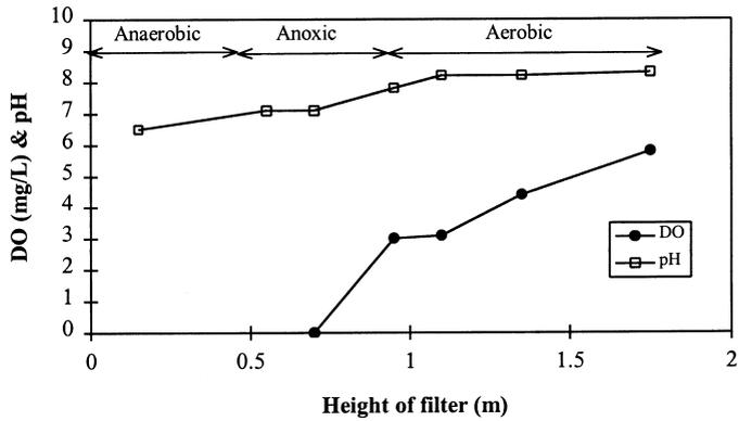
Figure 8 DO and pH profiles in the single combined filter
