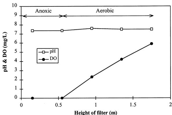
Figure 6 DO and pH profiles in the A/O filter
