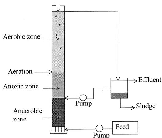
Figure 2 Schematic diagram of the single combined filter system
