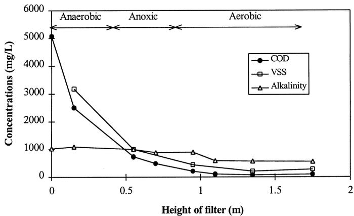
Figure 9 COD, VSS and alkalinity profiles in the single combined filter
