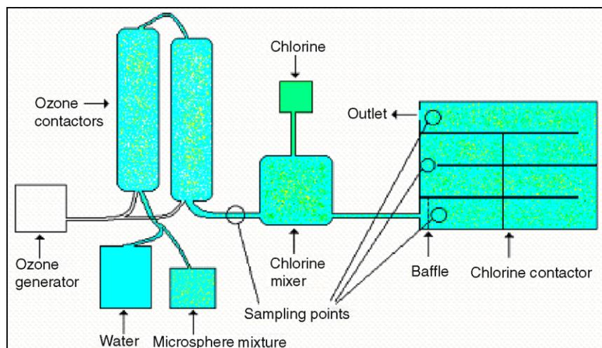
Figure 1 | Sequential disinfection of continuous-flow system.
