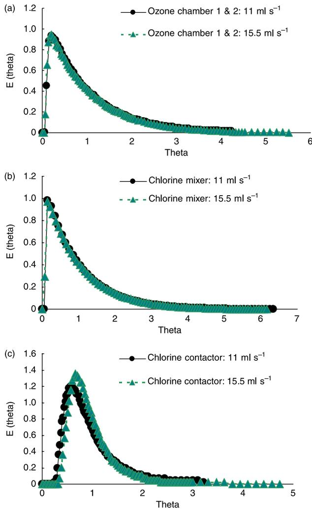
**Figure 2** | Residence time density functions for different parts of the sequential disinfection pilot system: (a) ozone chamber 1 and ozone chamber 2, (b) chlorine mixing chamber, (c) chlorine contactor.
