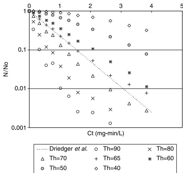
**Figure 4** | Microspheres inactivation with ozone (0.29 mg/L) at pH 7.5,  $20 \pm 2^\circ\text{C}$ , and for a duration of 90 min. Reference inactivation curve based on Driedger *et al.* (2000).
