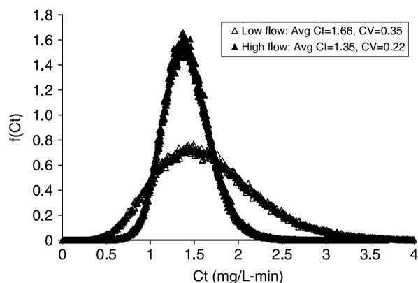
Figure 5 | Ozone effluent Ct distribution.
