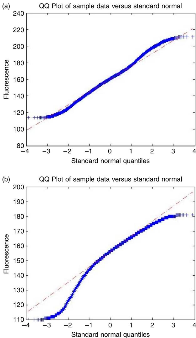
**Figure 3** | QQ-plot for microsphere fluorescence distribution data from the ozone contactor experiments: (a) Low flow, (b) High flow.
