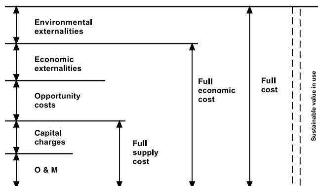
Figure 1 | Elements of the cost of water (modified from Rogers *et al.* 1998).
