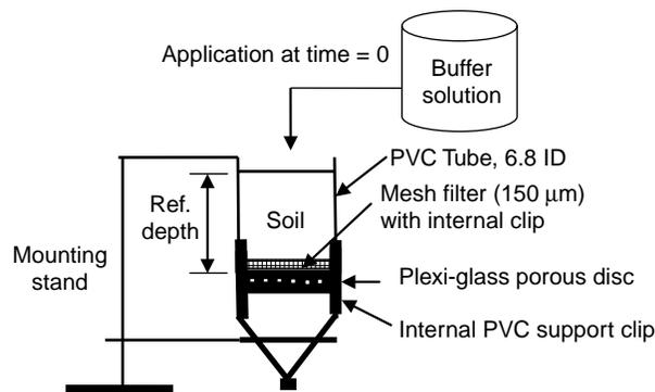
Figure 1 | Soil column setup for bacteria survival test.
