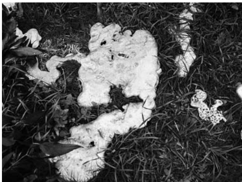
Figure 1. Metal puddle formerly a lawn mower, in the wake of the Black Saturday fires. April 2009. Photo by author
