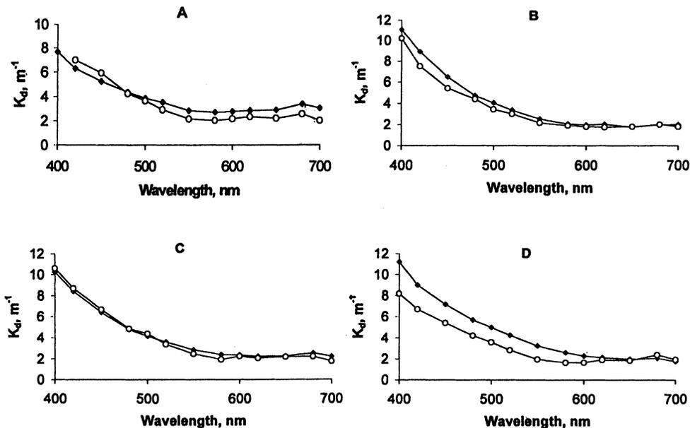
Fig. 3. Comparison of the spectra of  $K_{dc}$  (filled diamonds) with the corresponding spectra  $K_{dm}$  (open circles) for Lake Vörtsjärv: (a) September 1994, (b) June 1995, (c) August 1995, (d) August 1997.
