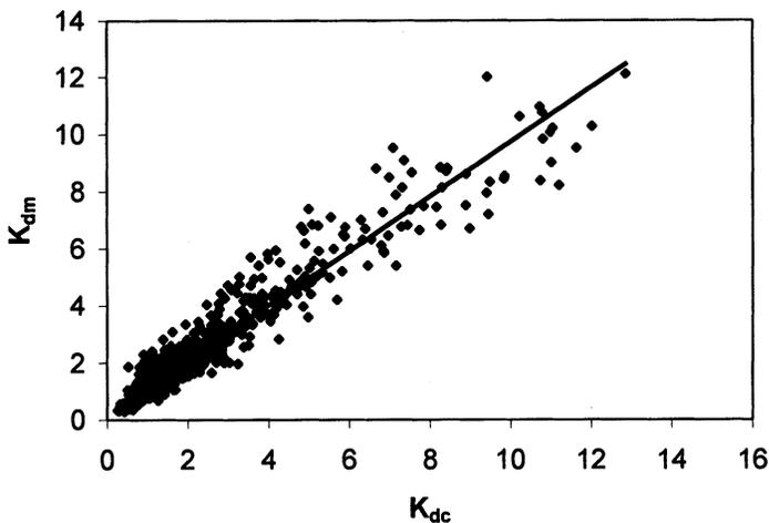
Fig. 4. Correlation between the values of the diffuse attenuation coefficient derived from the Hitachi U1000 measurements ( $K_{dc}$ ) and those obtained from underwater irradiance measurements ( $K_{dm}$ ). Data for 13 wavelengths between 400 and 700 nm for all lakes under investigation (Table 1) were used.
