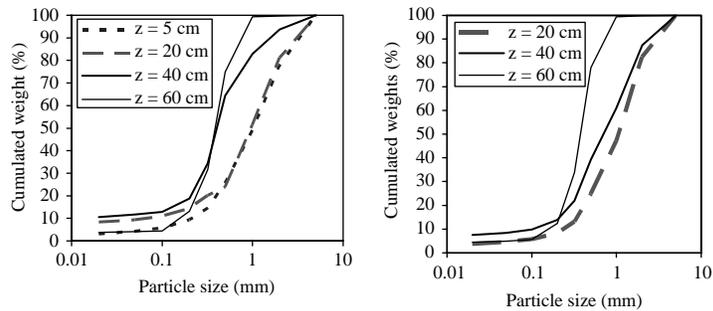
**Figure 4** Particle size distribution below the impounded area (left) and the water free area (right) at Vall-Llobrega
