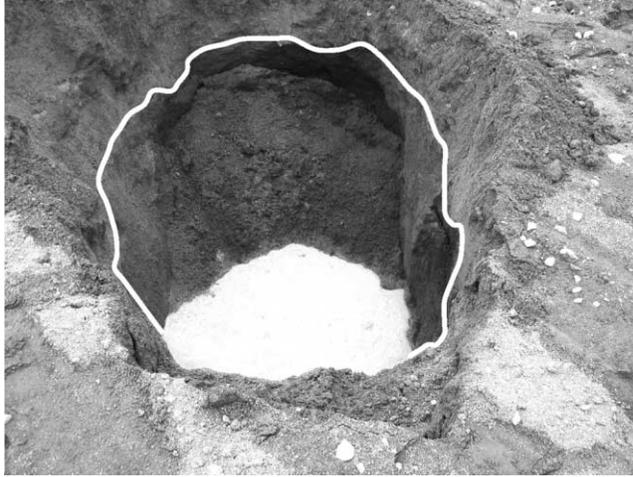
**Figure 6** Excavation in a bed clogged for misconstruction of the drainage outlet. The white line stresses the limit between the “clean” sand and the black anaerobic layer. The water of the saturated layer has invaded the bottom of the hole
