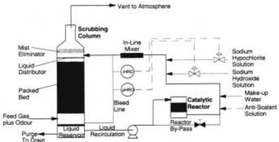
Figure 4 Simplified ODORGARD™ Process Flow Diagram (Higgins, 1998)
