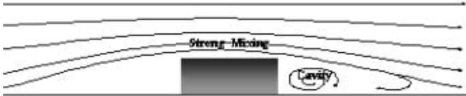
Figure 3 Simplified drawing of flow over a building
