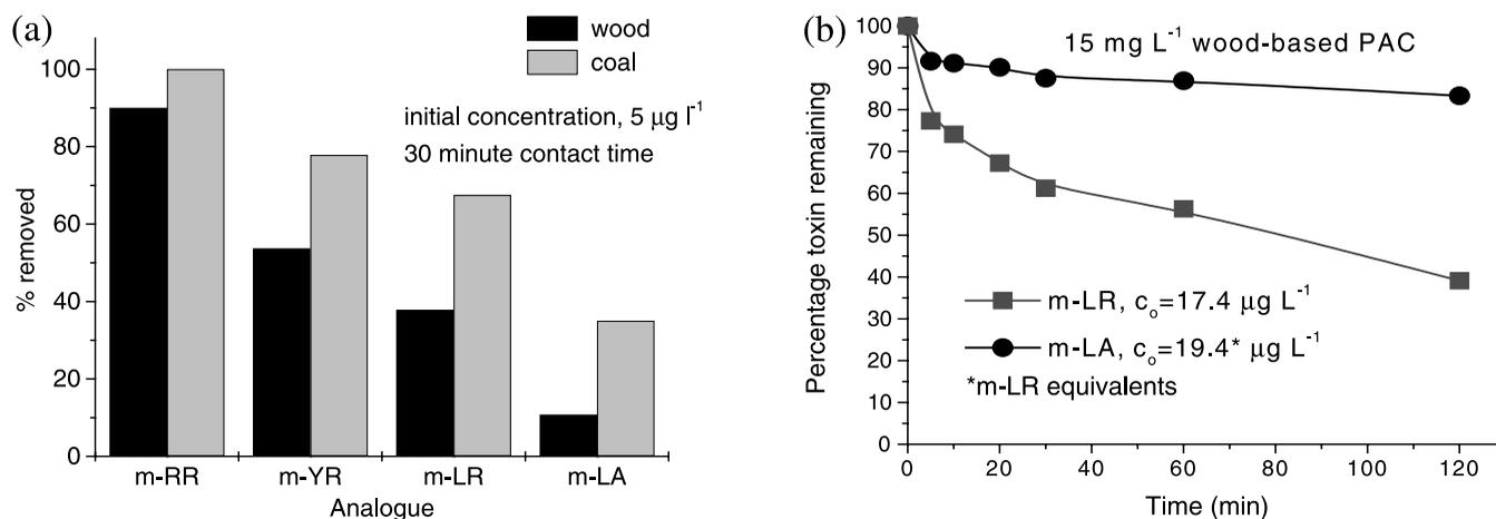
Figure 11 | Adsorption of microcystin variants (a) at 30 minutes contact time, (b) as a function of time.
