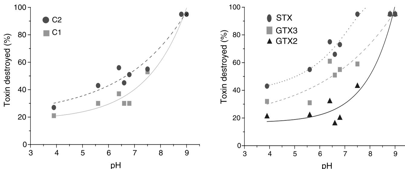
Figure 6 | Percentage saxitoxin destroyed by chlorine as a function of pH. Chlorine dose was sufficient to provide a  $0.5 \text{ mg l}^{-1}$  residual after 30 min.
