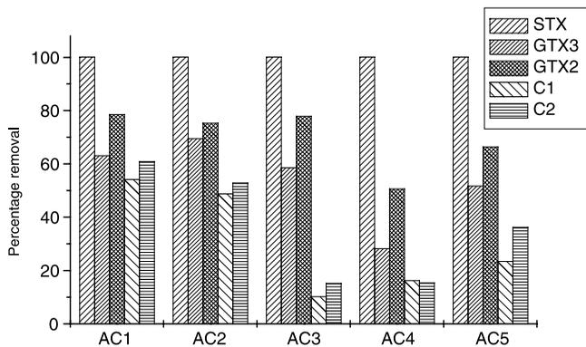
**Figure 12** | Percentage removal of saxitoxins for five activated carbons. Contact time=1 h, carbon dose=30 mg l<sup>-1</sup>.
