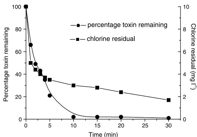
**Figure 5** | Percentage toxin remaining, and chlorine residual vs. time for a culture of *M. aeruginosa*.
