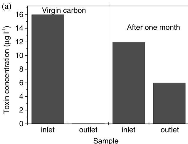
**Figure 13** | Microcystin removal across GAC filters, adsorption and biodegradation.
