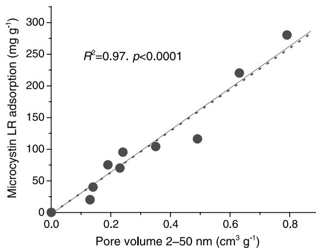
**Figure 10** | Microcystin LR adsorption vs. pore volume of activated carbons.
