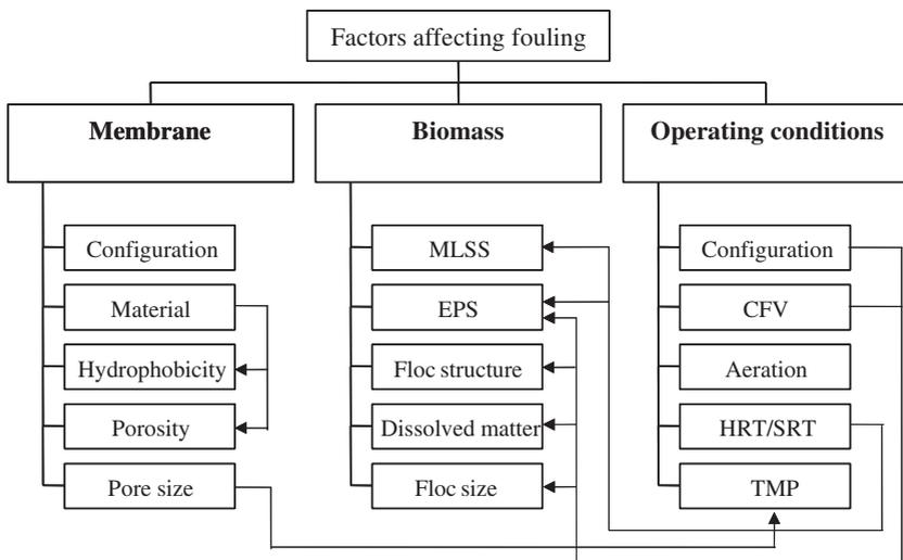
**Figure 1** Factors influencing membrane fouling in MBR process (taken from Chang *et al.*, 2002)
