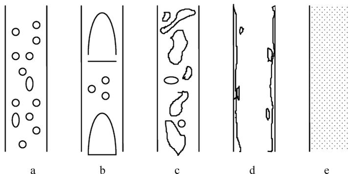
**Figure 3** Flow regimes for two-phase flow; (a) bubble flow, (b) slug flow, (c) churn flow, (d) annular flow, and (e) mist flow
