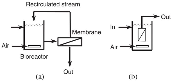
**Figure 2** (a) Sidestream, and (b) submerged MBRs
