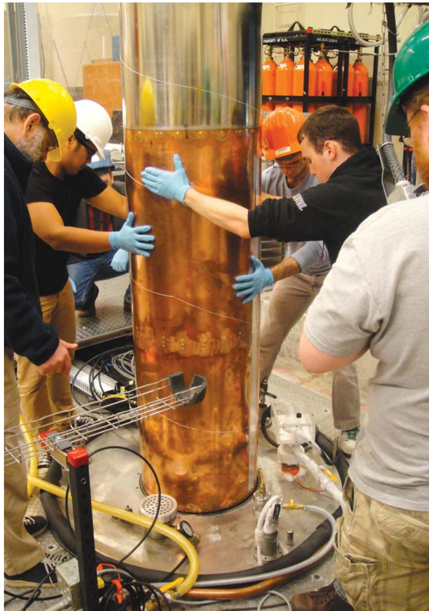
MEMBERS OF THE AXION DARK MATTER EXPERIMENT lower the deep cryogenic detector into the bore of a superconducting magnet. Shown are ADMX lead scientist Leslie Rosenberg (yellow hat), graduate students Nick Du (white hat) and Michael Hotz (green hat), and Cliff Plesha (no hat) and another undergraduate (orange hat), all of the University of Washington.
