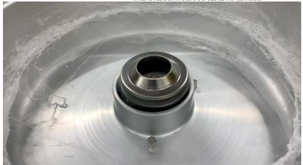
THIS COTTON CANDY MACHINE (diameter 70 cm) was retrofitted to make a high-quality filter material for face masks. The technique could enable inexpensive, local fabrication, especially in less developed regions of the world.
