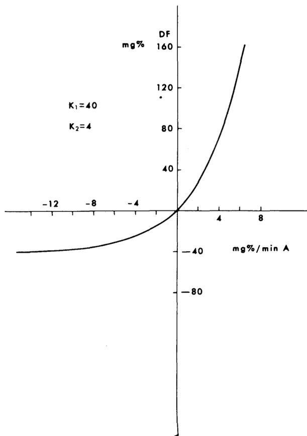
FIG. 3. Control algorithm relating the difference factor DF to the computed rate of change of blood sugar.
