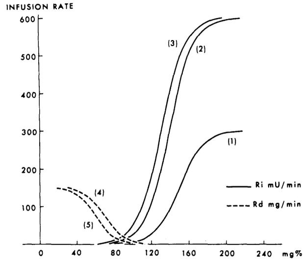
FIG. 2. Control algorithms relating insulin and dextrose infusion rates to projected blood glucose concentration. Curve parameters  $M, S, B$  are as follows: (1) 300, 0.04, 150; (2) 600, 0.04, 140; (3) 600, 0.04, 130; (4) 150, 0.05, 70; (5) 150, 0.05, 60.
